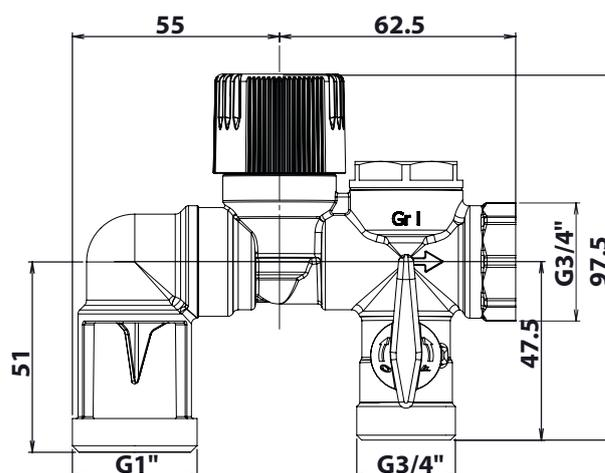
■ SIÈGE EN TÉFLON ADAPTÉ AUX EAUX CALCAIRES
